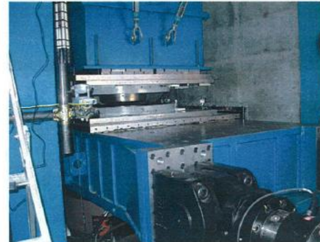
Figure 14. ALGAPEND APS 9100/1200-5 # 2 testing
